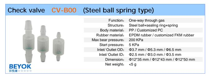
BEYOK CV-B/D/H/N series one-way valve/check valve provides one-way check function for air pipelines to prevent reverse flow of air/water in other directions. The structure includes steel ball spring type, diaphragm spring type, diaphragm high-pressure type, and diaphragm pressureless structure. It is an important component for ozone generators, household appliances, medical equipment, and other products to prevent damage caused by backwater.
