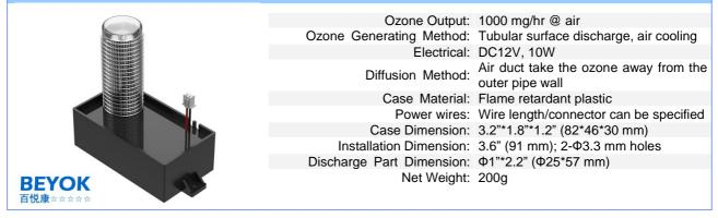
The FQA- series of BEYOK ozone generator air disinfection tube type ozone module uses glass/ceramic tube along the surface discharge body, including the ozone tube and ozone driving circuit. Once given power, ozone can be output and directly dispersed into the air, suitable for various sizes of household appliances and ventilation systems and other air disinfection occasions.
