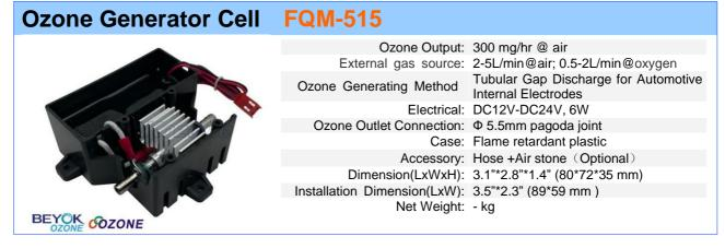
The FQM-5 series of BEYOK split-tube ozone module adopts stainless steel rod/titanium rod/aluminum rod to make the inner electrode gap discharge ozone core discharge body, including the split design of ozone generating tube and ozone driving circuit, and is connected to another Air pump or other air source can provide efficient and stable ozone output as long as it is connected to the power supply, and the split installation is flexible.
