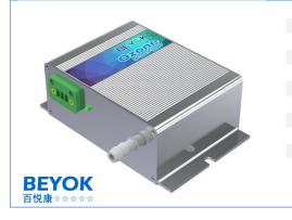
Ozone Output:300-500 mg/hr @ O2External gas source:0.5L/min@oxygenOzone Generating MethodCorona DischargeElectrical:AC220V-AC110V-DC12V, 6WOzone Outlet Connection: $\Phi7mm$  pagoda jointCase:Aluminum profileOzone Adjustable:Can not be adjustedDimension (LxWxH):3.8"\*1.6"\*2.9" (96\*40\*73 mm)Installation Dimension (LxW):4.3" (110 mm)Net Weight:- kg
