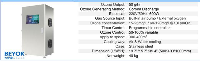
The GQO-A series of BEYOK skid-mounted ozone generators can mix ozone into water to destroy bacteria, purify air and eliminate peculiar smell. They are suitable for food factory assembly lines, restaurants, and refrigerated storages, etc. Connect to the external oxygen source will provide a higher concentration of ozone.
