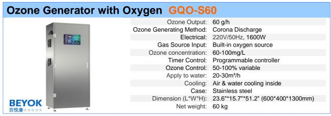
The GQO-S series of BEYOK skid-mounted ozone generators have perfect automatic ozone production systems including oxygen source system, ozone system, gas-water mixing system, cooling system and automatic control system, can destroy bacteria, purify air and eliminate peculiar smell automatically. They are suitable for large food processing plants, canteen, sewage treatment, etc.
