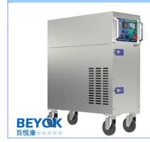
Ozone Output:10 g/hOzone Generating Method:Corona DischargeElectrical:220V/50Hz, 800WFeed gas:Built-in oxygen sourceOzone concentration in water:1-3 ppmTreat water flow:0.5-1.0 m3/hTimer Control:Programmable controllerOzone Control:50-100% variableWater Connection:3/4-in, 3/4-inCase:Stainless steelDimension (L\*W\*H):31.5"\*13.4"\*38.3" (800\*340\*972mm)Net weight:60 kg
