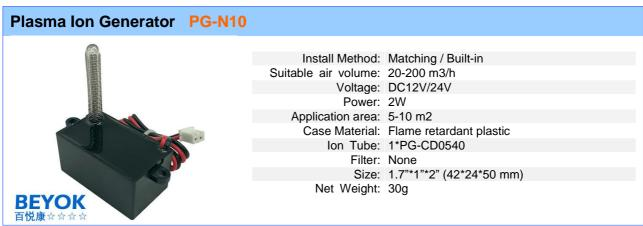
BEYOKozone PG-N series plasma generator (Plasma Generator) uses a high-voltage electric field to convert the electrons in the atomic particles in the air into charged ions to simulate the air environment in the natural forest, and interact with bacteria and bacteria in the air. Viruses, pollutants and other impact ionization to decomposition and elimination, significantly improve indoor air quality, effectively and quickly remove and decompose various harmful pollutants.
