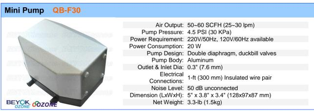
BEYOKozone Mini Pump Series use a unique linear motion design that has the capability of over 18,000 hours of continuous maintenance-free operation. They are compact, very quiet, highly reliable and inexpensive.
